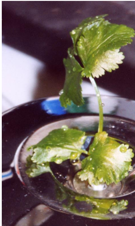
Figure 2.8: Photograph of a coriander leaf in the pressure chamber. Water is being forced out of the stomata on the leaves, clearly illustrating the elevated pressure to which it is being subjected.
